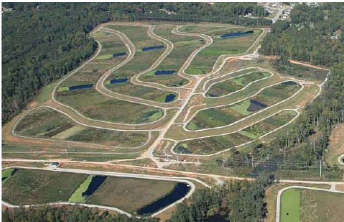
Tertiary treatment wetlands reduce the amount of nutrients discharged into local waterways. Photo presented to the Water Resources subcommittee, 2008.
